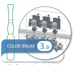
Color Break on the ampoules or rings codification.
