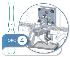
Point and cut to indicate the ampoule break, controlled by a camera.
